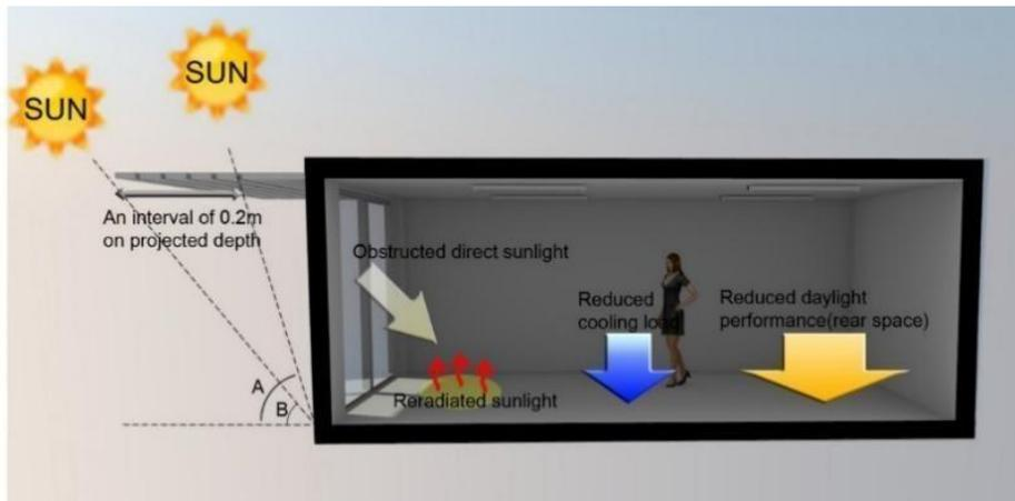
**Figure 2:** Horizontal louver conceptual diagram.
