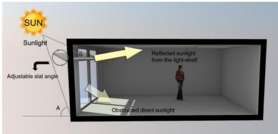
**Figure 4:** Type-B light shelf conceptual diagram.
