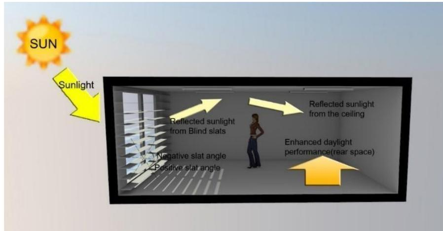
**Figure 1:** Horizontal blind conceptual diagram.
