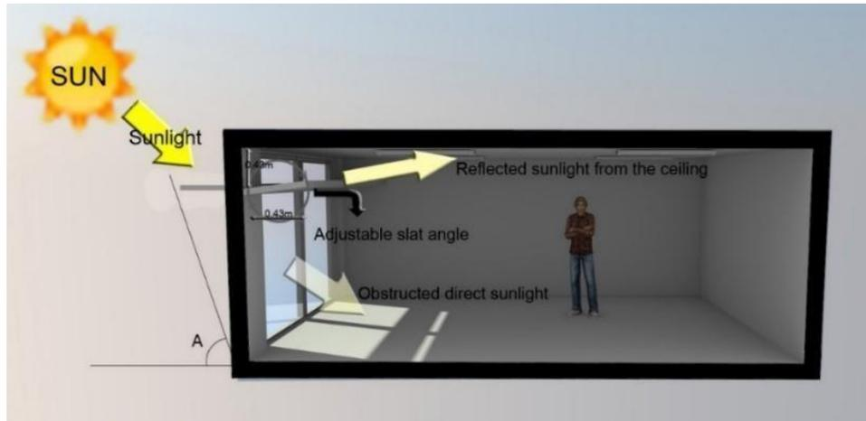
**Figure 3:** Type-A light shelf conceptual diagram.
