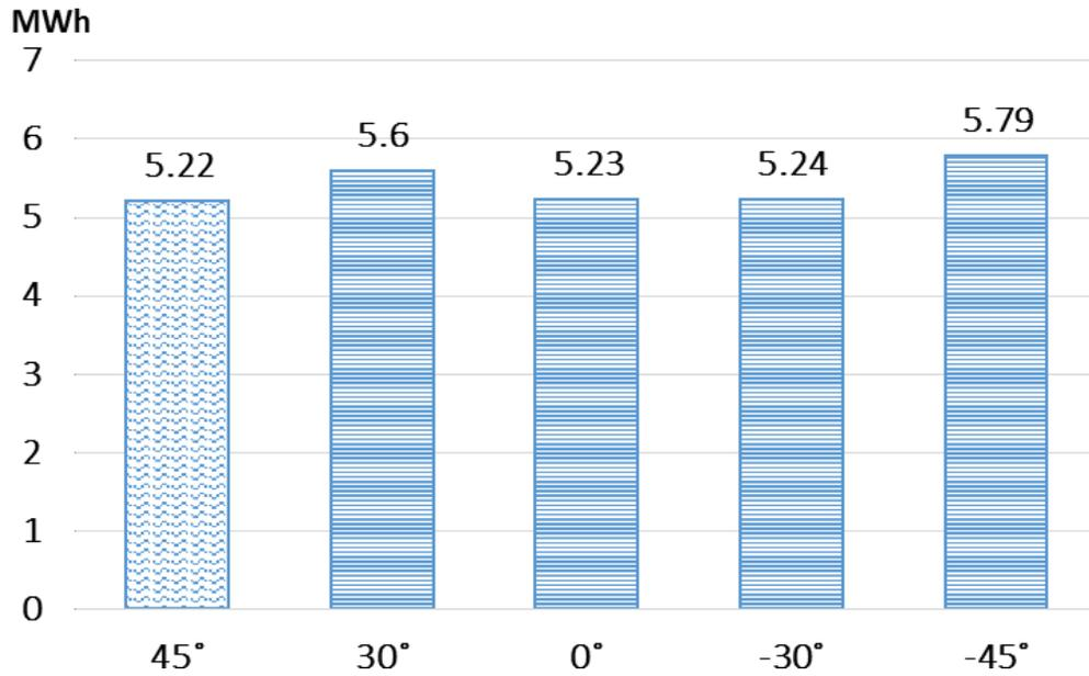
**Figure 7:** Annual cooling load based on slat angles of a horizontal blind system.
