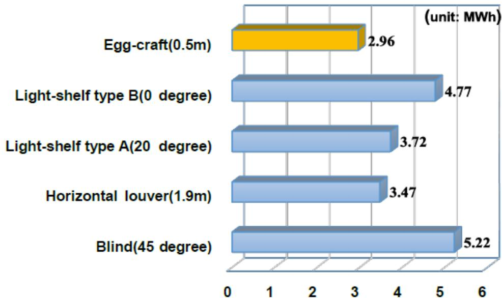
Figure 12: Comparative analysis of various shading devices based on annual cooling load.
