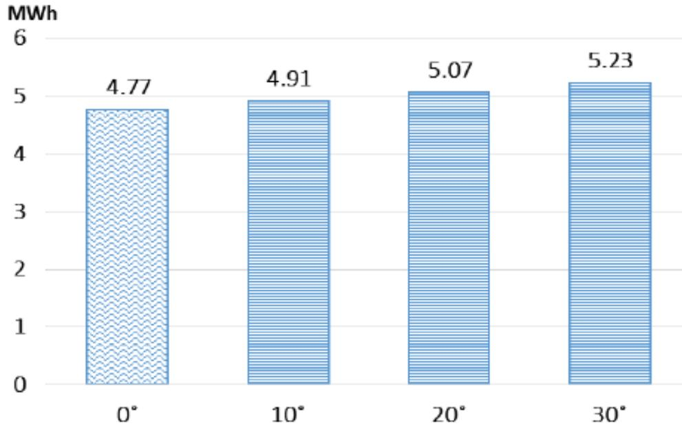
Figure 11: Annual cooling load performance of the egg craft system based on projection length.
