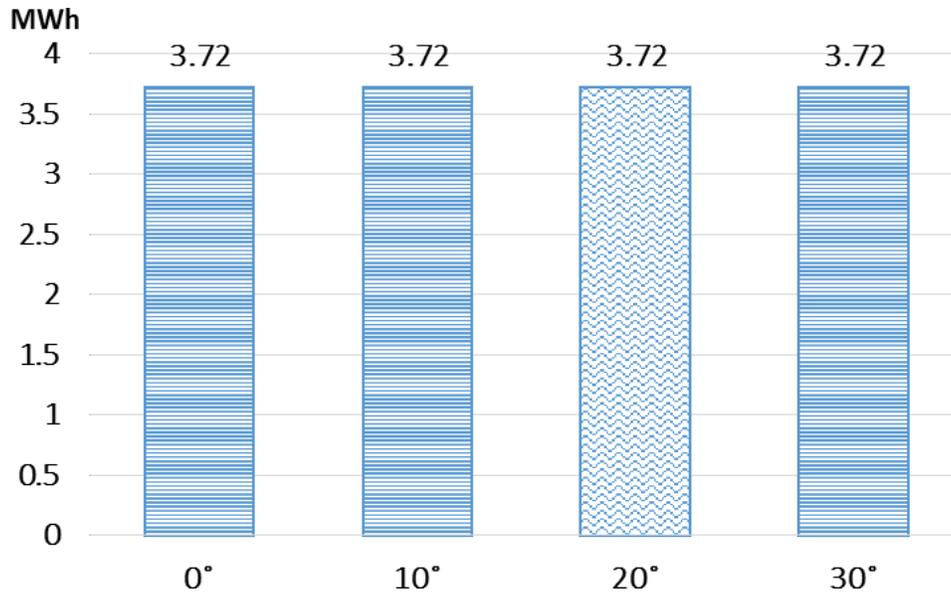
**Figure 9:** Annual cooling load performance of the light-shelf Type-A based on slat angles.
