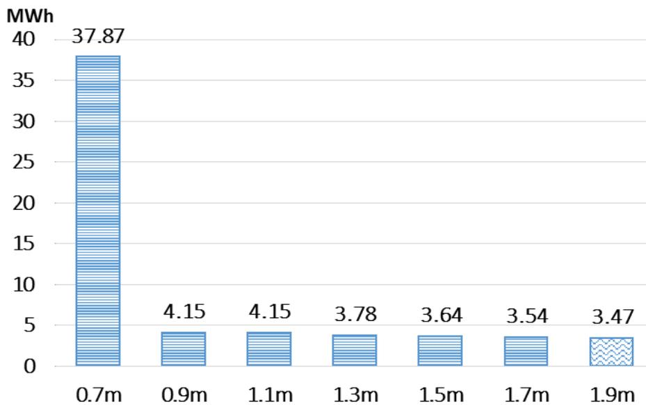
**Figure 8:** Annual cooling load based on the projection-length of the horizontal louver.
