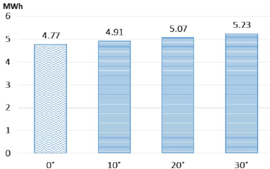
**Figure 10:** Annual cooling load performance of the light-shelf Type-B based on slat angles.
