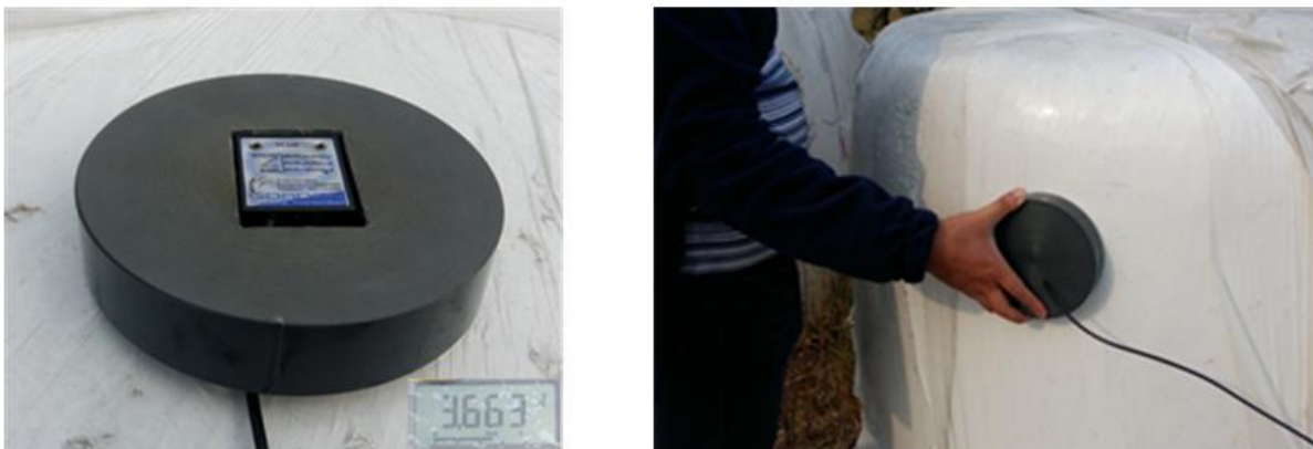
Figure 3: Moisture content measurement test using electrical resistance method.
