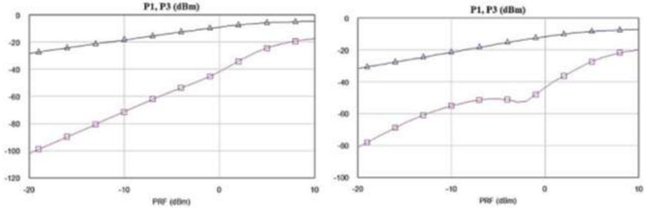
**Figure 9:** Intermodulation products at the inductor values of 10 nH (left) and 4 uH (right). The infinite IP3 phenomenon is clearly shown in the right Figure. Notations: Triangles – first order, squares – third order intermodulation products (AWR analysis).
