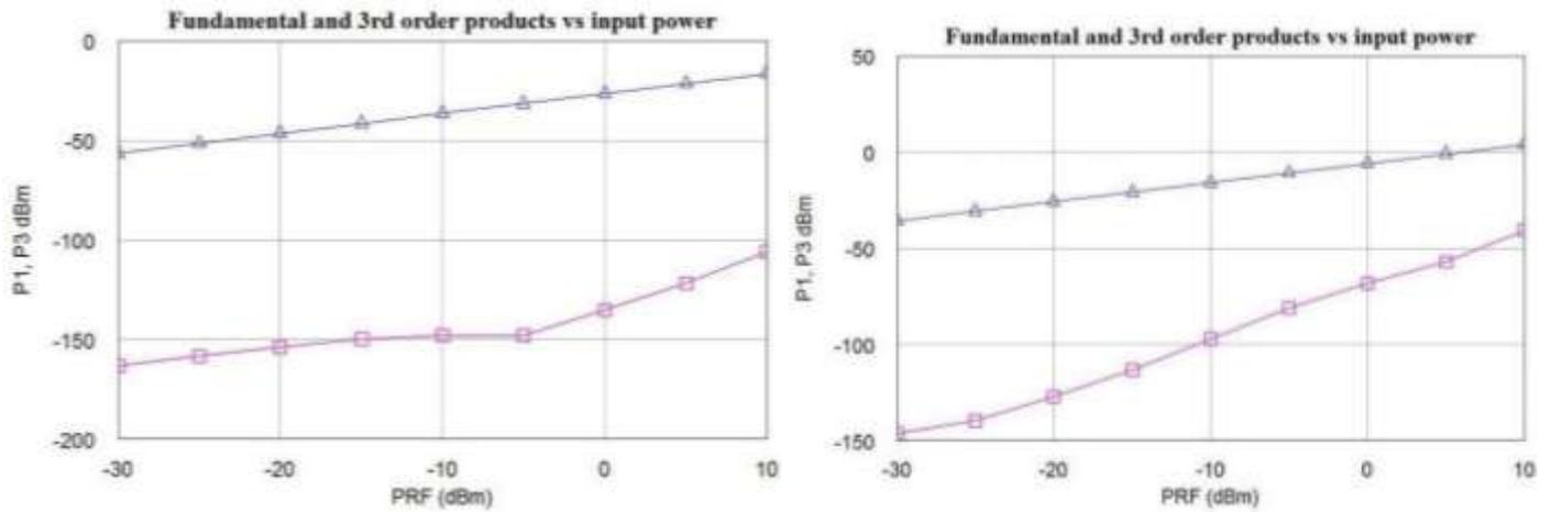
**Figure 5:** Intermodulation analyses for the Gilbert mixer (Figure 3). Left: Transformer self-inductances are 0.4 uH, right: 4 uH. As expected. Transformer parasitics are neglected.
