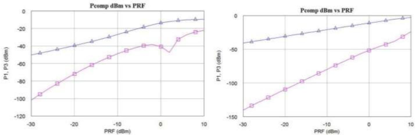
**Figure 6:** Intermodulation analyses for the half H mixer (Figure 4 Left: Transformer self-inductances are 0.15uH, right: 1.5uH. As expected. Transformer parasitics are neglected.
