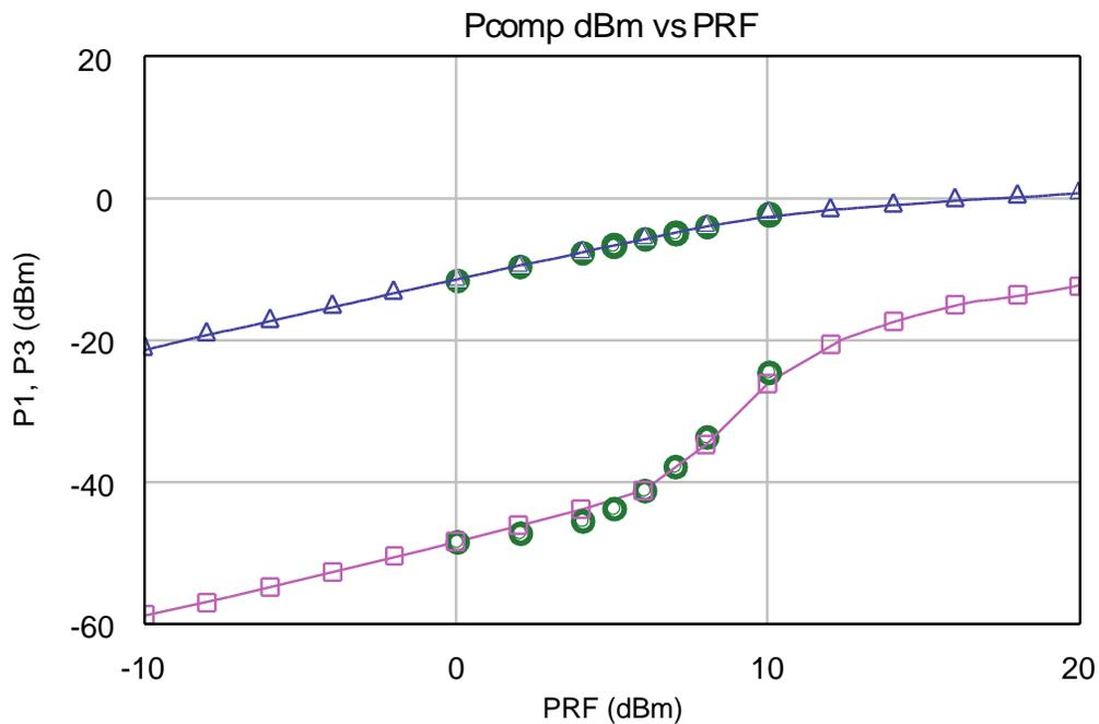
**Figure 4:** Intermodulation vs. input power for the diode half H mixer. Infinite IP3 phenomenon is observed here as well. Notations: Triangles – first order, squares – third order intermodulation products (AWR analysis), circles – measurements.
