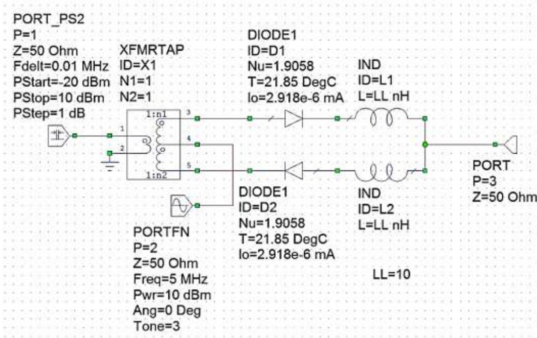
Figure 7: Circuit diagram of the two-diode mixer, a plot from the analysis program AWR.
