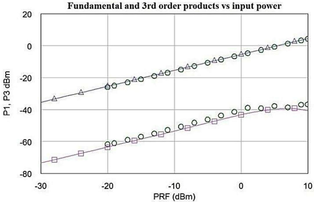
**Figure 3:** Power of the 1<sup>st</sup> and the 3<sup>rd</sup> order intermodulation of a modified Gilbert mixer vs. input power. The two curves can be approximated well by two parallel lines. Parallel means that the point of intersection is in the infinity. Thus, this is called as infinite IP3 phenomenon. Notations: Triangles – first order, squares – third order intermodulation products (AWR analysis), circles – measurements.
