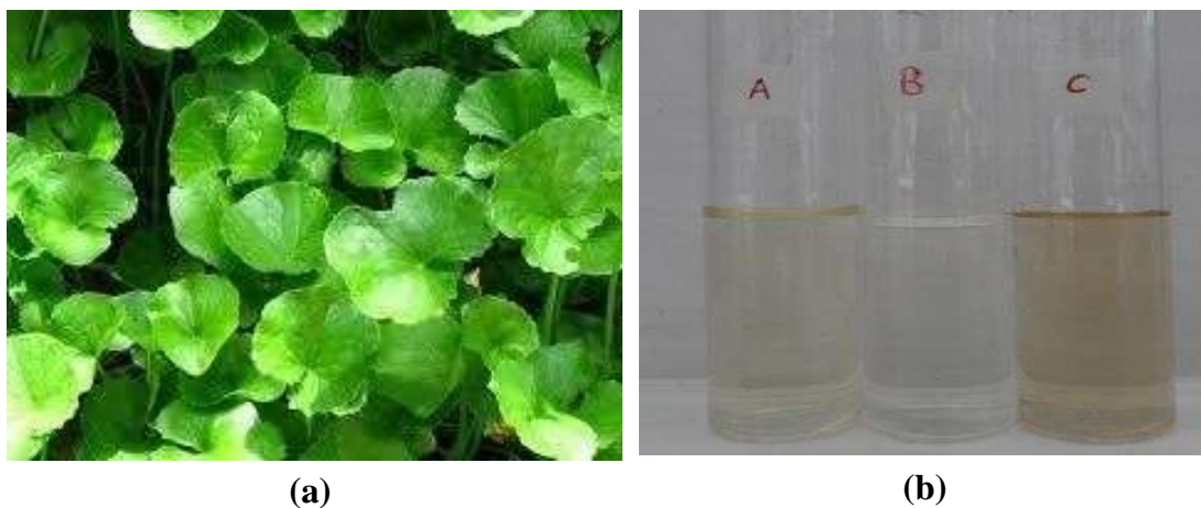
Figure 1(a): Centella asiatica plant (b) Tube A- contain Centella asiatica leaf extract, Tube B- contain \text{AgNO}_3 solution, Tube C- contain light brown colored silver nanoparticles solution.
