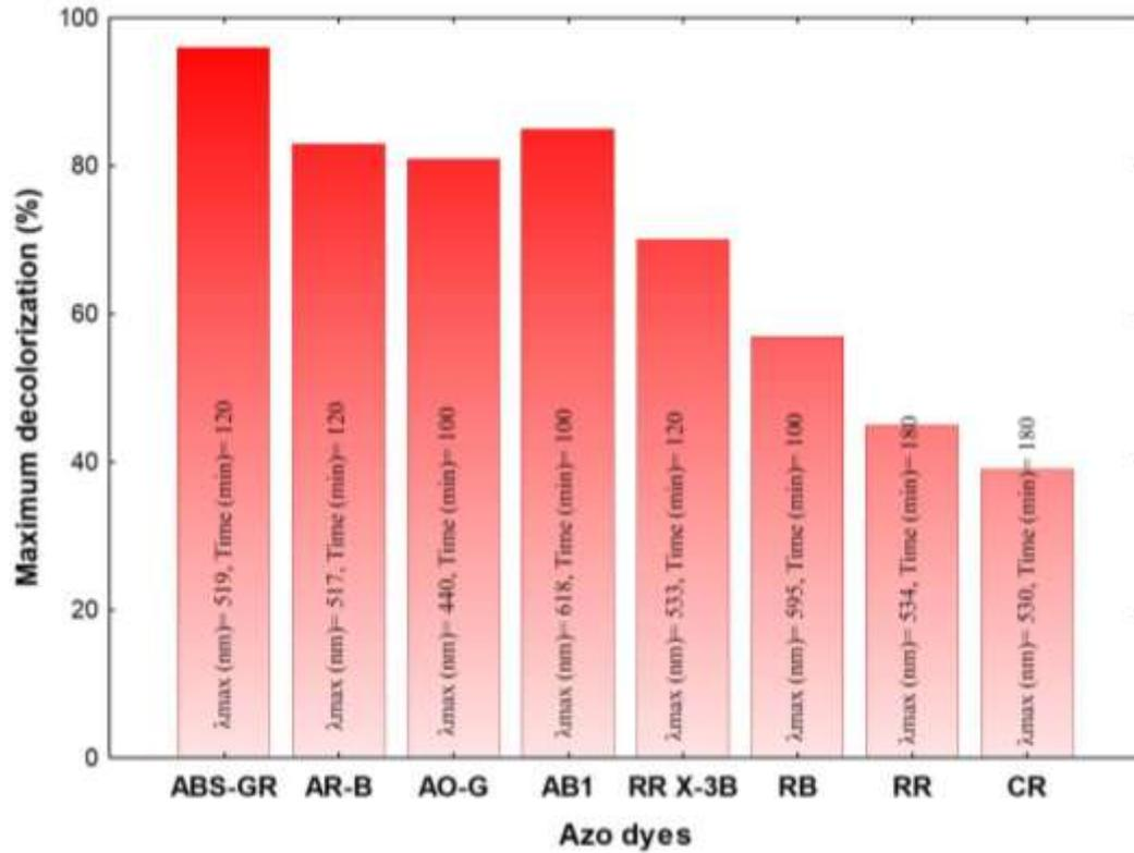
**Figure 10:** Decolorization of azo dyes (50 mg/L) by bio-AuNPs. Acid Brilliant Scarlet GR (ABS-GR), Acid Red B (AR-B), Acid Orange G (AO-G), Acid Black 1 (AB1), Reactive Red X-3B (RR X-3B), Reactive Black (RB), Reactive Red (RR), Cation Red (CR).
