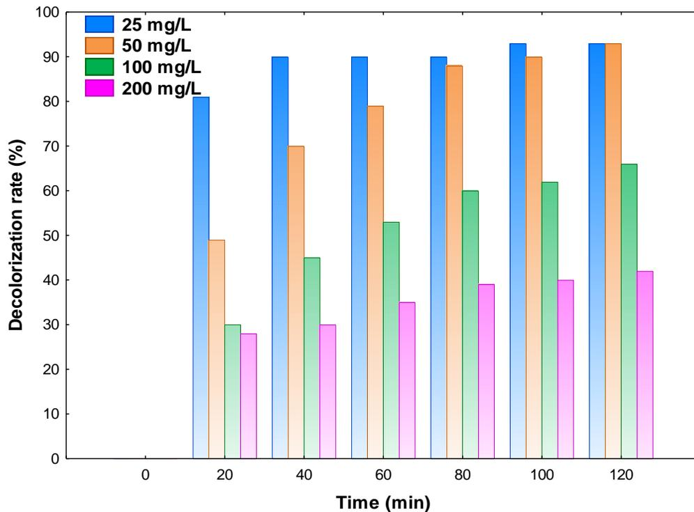
**Figure 11:** Effects of initial concentration (25, 50, 100, 200 mg/L) of Acid Brilliant Scarlet GR on decolorization.
