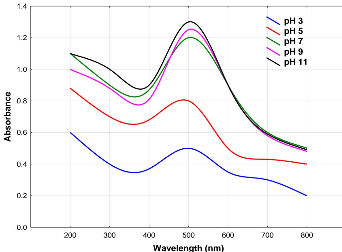
**Figure 9:** UV-Vis spectra of the dispersed AuNPs synthesized under different conditions of pH (3, 5, 7, 9, 11) in reaction solutions.
