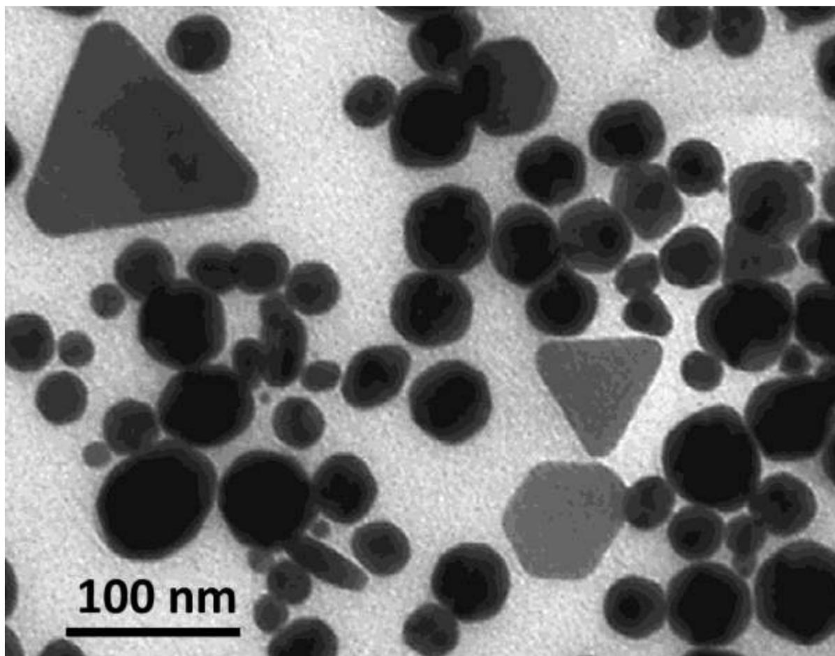
**Figure 6:** The TEM image of AuNPs synthesized by strain *M. indicus* CBS 226.29 ET.
