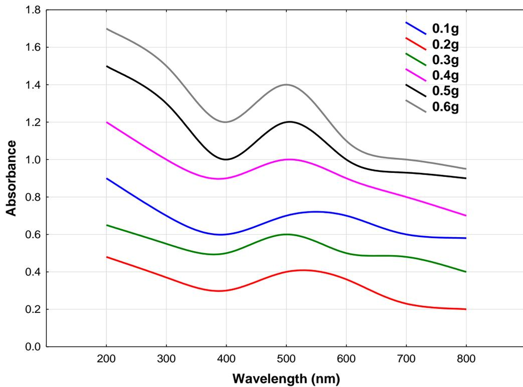
**Figure 8:** UV-Vis spectra of the dispersed AuNPs synthesized under different concentrations of strain *M. indicus* CBS 226.29 ET biomass (0.1, 0.2, 0.3, 0.4, 0.5, 0.6 g) in reaction solutions.
