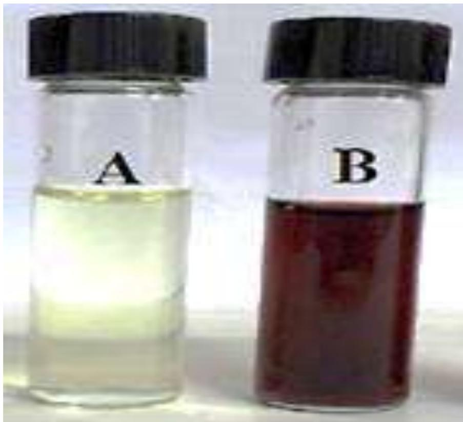
**Figure 4:** The pale yellowish reaction mixture A changed to violet color B, indicating the formation of gold nanoparticles.
