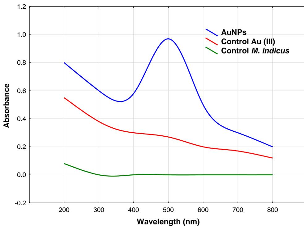
**Figure 5:** UV-vis spectra of the dispersed AuNPs synthesized by strain *M. indicus* CBS 226.29 ET after 40 h incubation, HAuCl<sub>4</sub> solution, and control strain *M. indicus* CBS 226.29 ET.
