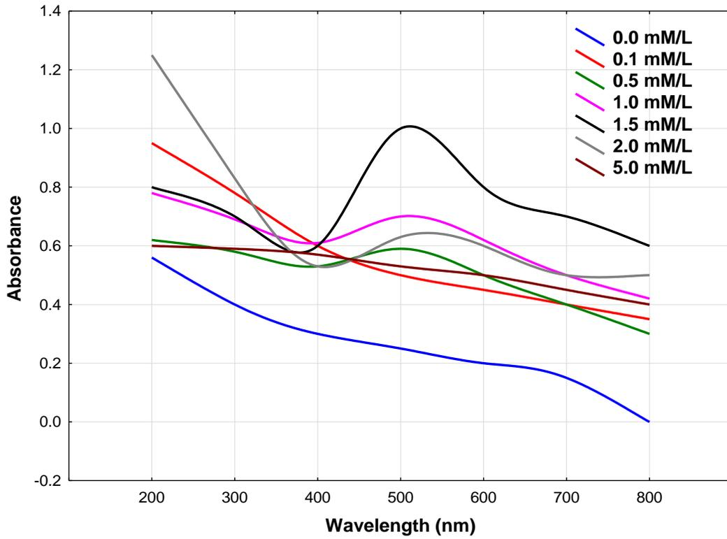
**Figure 7:** UV-Vis spectra of the dispersed AuNPs synthesized under different concentrations of HAuCl<sub>4</sub> (0.1, 0.5, 1.0, 1.5, 2.0, 5.0 mM) in reaction solutions.
