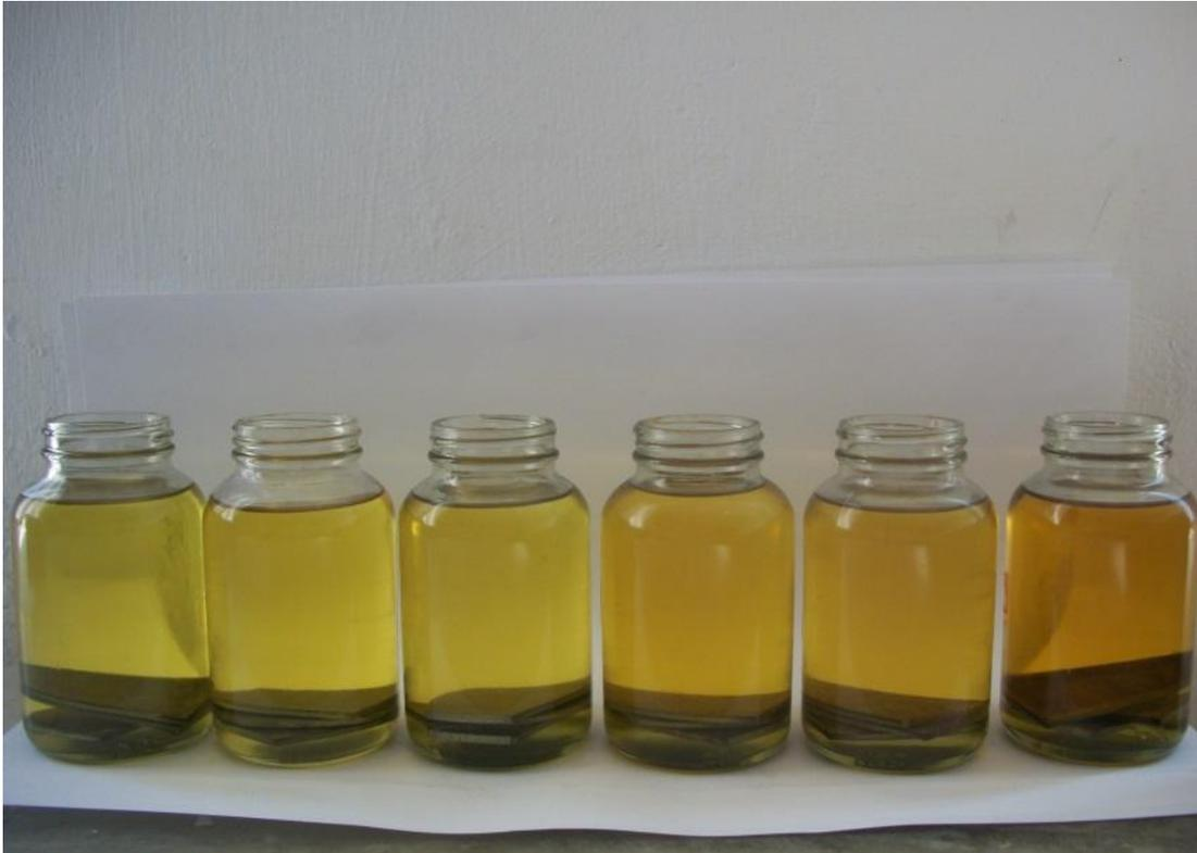
**Figure 3.** The sedimentation of biodiesel in petro-diesel of pure petro-diesel (left), 5% biodiesel, 10% biodiesel, 20% biodiesel, 50% biodiesel and 100% biodiesel (right).
